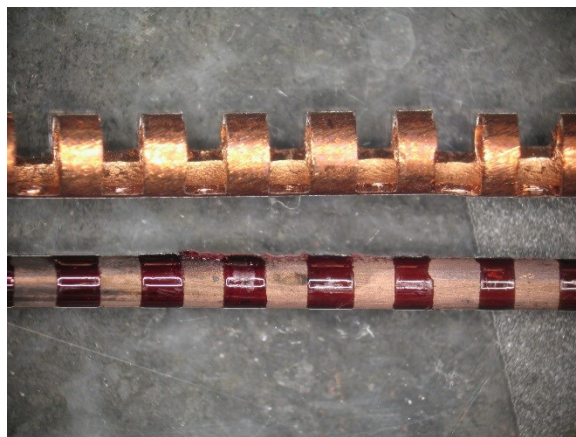
Figure 2.12 Preliminary 3D Lithography Stencil and Resulting Structure.
