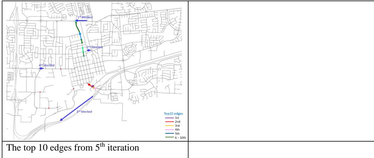
Figure 4.3 Changes in traffic flow with traffic light delay with sequential removal of critical edge. At the end of each iteration the critical edge is removed.
