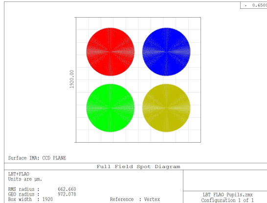
Fig. 8: Geometrical re-imaging at the FLAO PWFS pupil plane. The square side is in microns and corresponds to 80 pixels (with size equals 0.024 mm). According to the FLAO design (Esposito et al. 2003), single pupil size is 30 pixels and the distance between adjacent pupils is 36 pixels.
