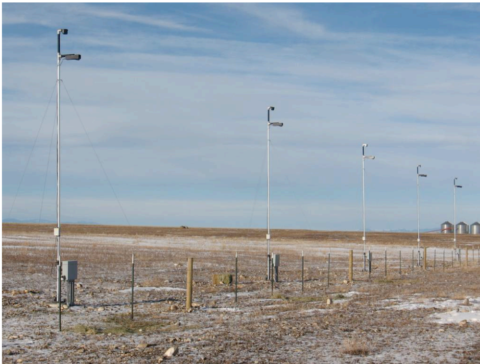
Figure 5. The infrared cameras that monitor animal movements in the enclosure (Photo: Marcel Huijser, WTI/MSU).
