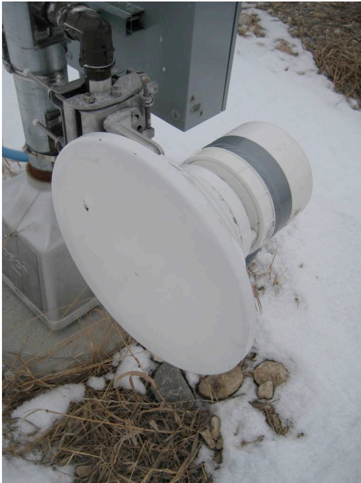
Figure 6. The receiver of the third generation break-the-beam system manufactured by ICx Radar Systems. Note: the transmitter looks similar to the receiver.
