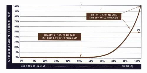
Stedman says: the way around the accuracy problem is to flag only those cars with very high emission readings on the remote sensor. This guards against "false fails." EPA replies: Yes, but a high cutpoint will allow some gross emitters to escape detection.
