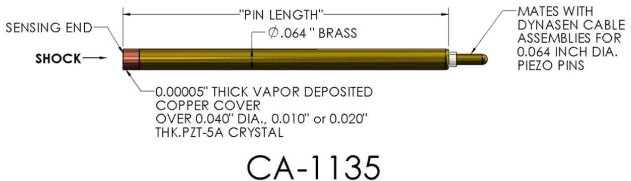
Figure D.10: Drawing of the piezoelectric sensor (CA-1135) used to measure shock speed on the high-enthalpy shock tube facility. The sensors, as well as this drawing, are obtained from Dynasen, Inc. located in Goleta, CA.
