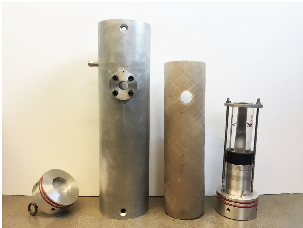
Figure 9.4: Parts manufactured and tested for the high-pressure hybrid-propellant combustion chamber. From left to right: end cap with graphite nozzle, combustion chamber with optical access for thermochemistry measurements, fiberglass phenolic insulation, and the current assembly described in Ch. 6 with a burnt PMMA fuel grain
