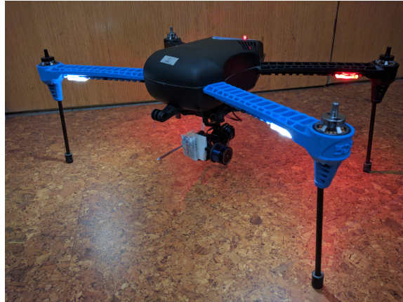
Figure 3.7: An IRIS+ with the airspeed sensor attached to a camera gimbal.
