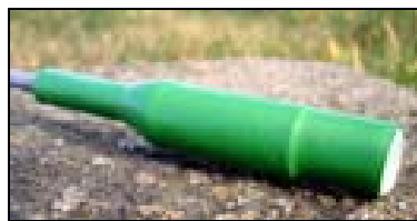
Figure 4.1: People counter with single pyroelectric sensor (Eco-Counter)
