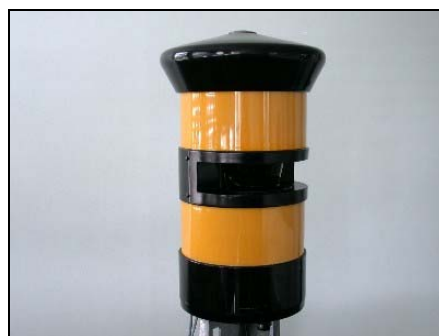
Figure 6.1: Horizontal scanning configuration (Lottraffic with Sick laser scanner)
