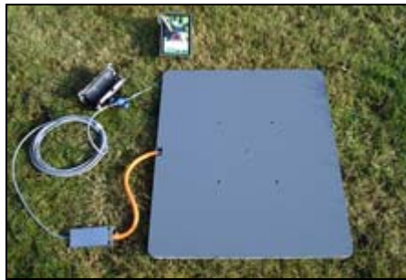
Figure 5.1: Piezoelectric pad counter (Eco-Counter)
