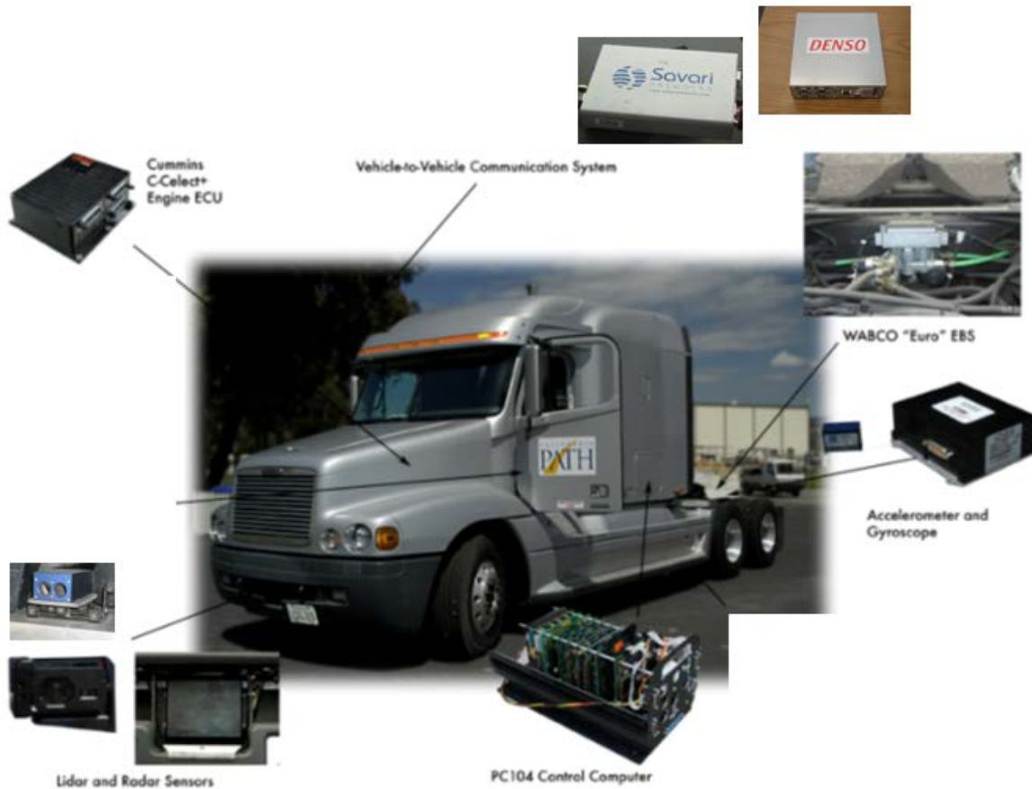
Figure 2.2 Sensors and Actuators Installed on Three Trucks
