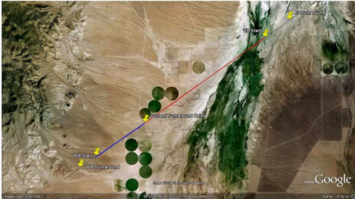
Figure 2.4 SR722 in Austin Nevada. The Red section is almost flat; the Blue Section contains a hill with Grade Levels A, B, and C as defined in Table 2.1.
