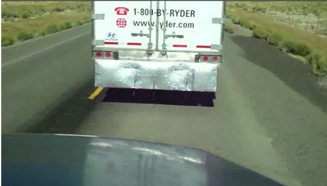
Figure 5.1. Reflector to help lidar and radar detection behind and underneath the trailer.
