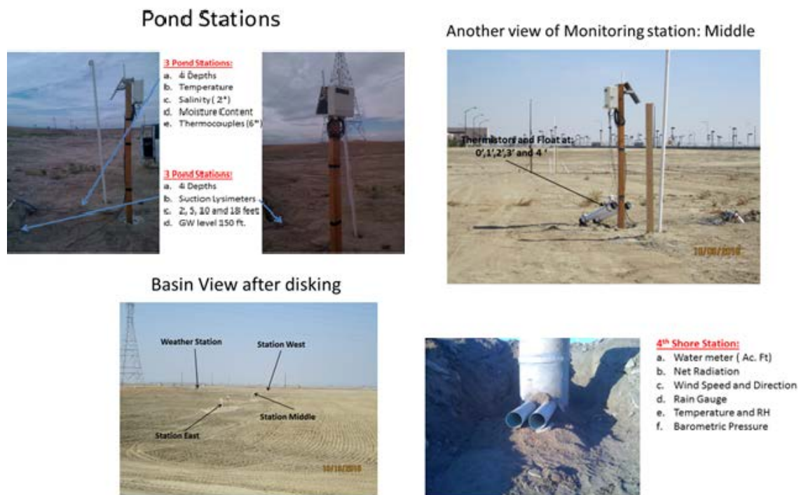
Figure 6: Instrumentations setup for basin 3, the three pond instrumentation location at were West, Middle, and East as shown in the bottom left image. The image on the bottom right show the modified standpipe assembly for measurement of water inputs.
