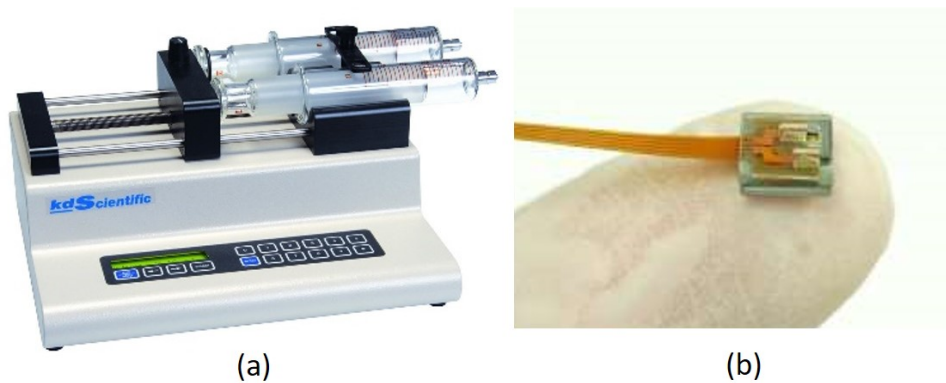
Figure 9.1: A two-channel syringe pump [129](a) and a stainless steel piezoelectric micropump [130] (b).
