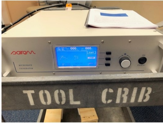
Figure 4.5: SAIREM GMS200W Microwave Generator was used to deliver 50 W microwave power into the interstitial ablation antenna. Input and reflected power were recorded from the panel with 5 seconds intervals.
