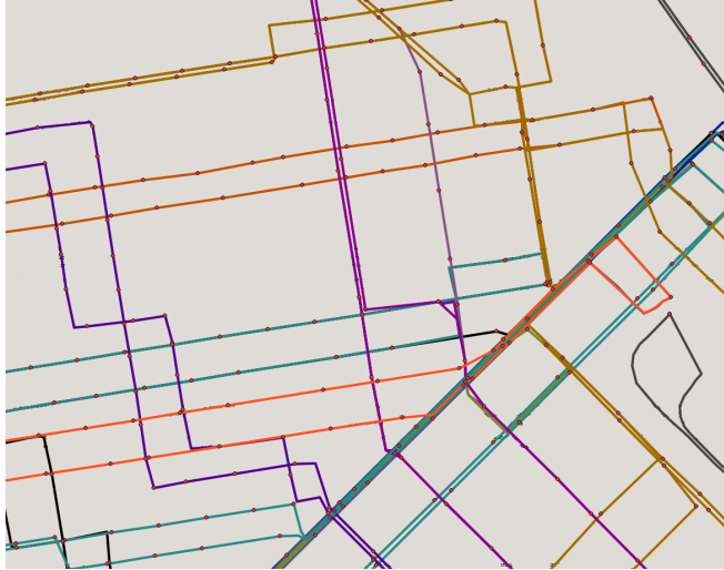
Figure 6: Example transit network structure built from open transit data with no link travel times defined.
