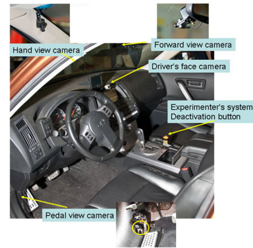
Figure 2: Vehicle interior with video camera locations shown
