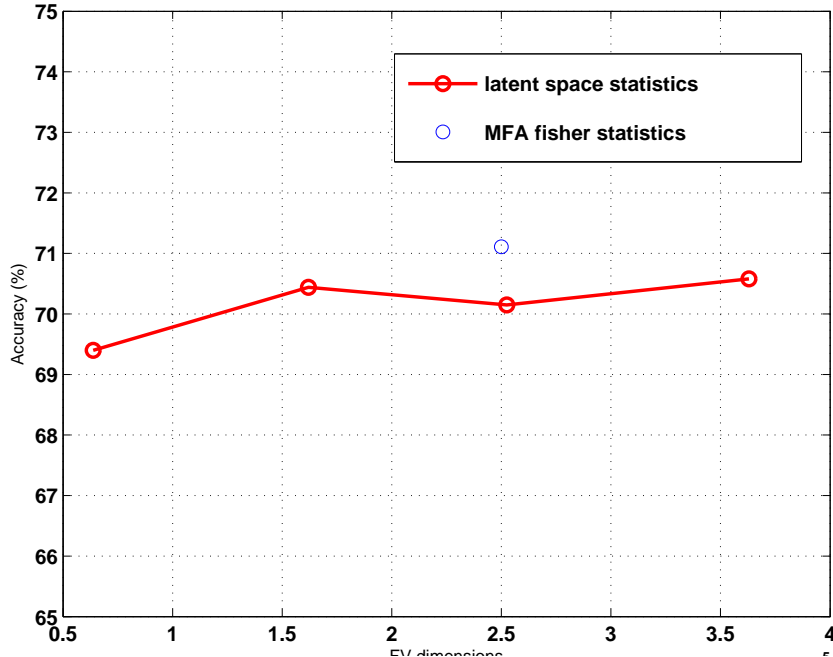
Figure III.1: Performance of Latent space statistics of (III.12) for different latent space dimensions. The accuracy of MFA-FS (III.14) for K=50 , R=10 included for reference.
