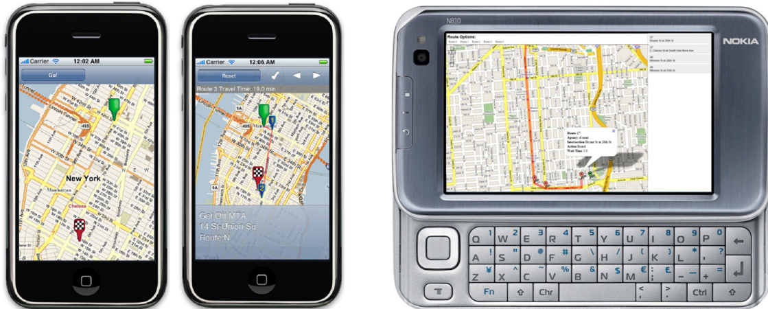
Figure 2: iPhone and web-browser implementation. Markers on screen indicate transfer points, and clicking on the markers or swiping the bar at the bottom of the screen reveals more information, such as the name/location of the stop and waiting times. The arrows on the top right of the touch screen can be used to toggle between different routes, while an information panel displays the total travel time for a selected route.
