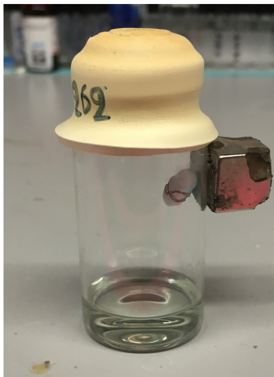
Figure 6.2: Photo of the reaction setup showing the stirbar with copper wire wrapped around it. The stir bar is magnetized to the side of the reaction vessel during the degassing step.
