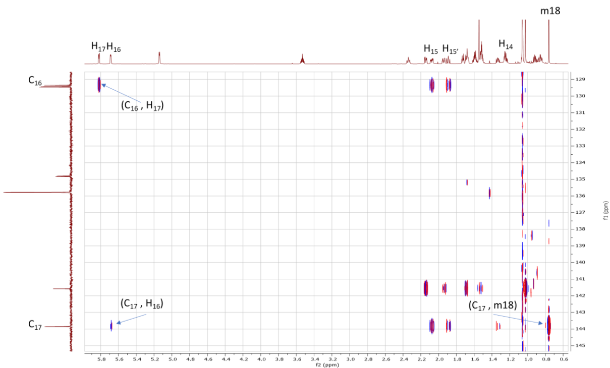
Figure 3.51D ^1\text{H} - ^{13}\text{C} HMBC Correlations in D ring for DHEA \text{C}_{17-16} Alkene PG (7a) ( \text{C}_{16} - \text{C}_{17} )
