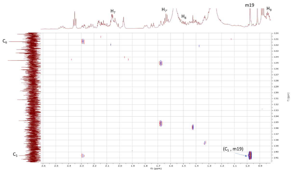
Figure 3.65D ^1\text{H} - ^{13}\text{C} HMBC Correlations in B ring for DHEA \text{C}_{17} -(R)- \text{N}_3 -MAN Product (29) ( \text{C}_5 - \text{C}_6 )
