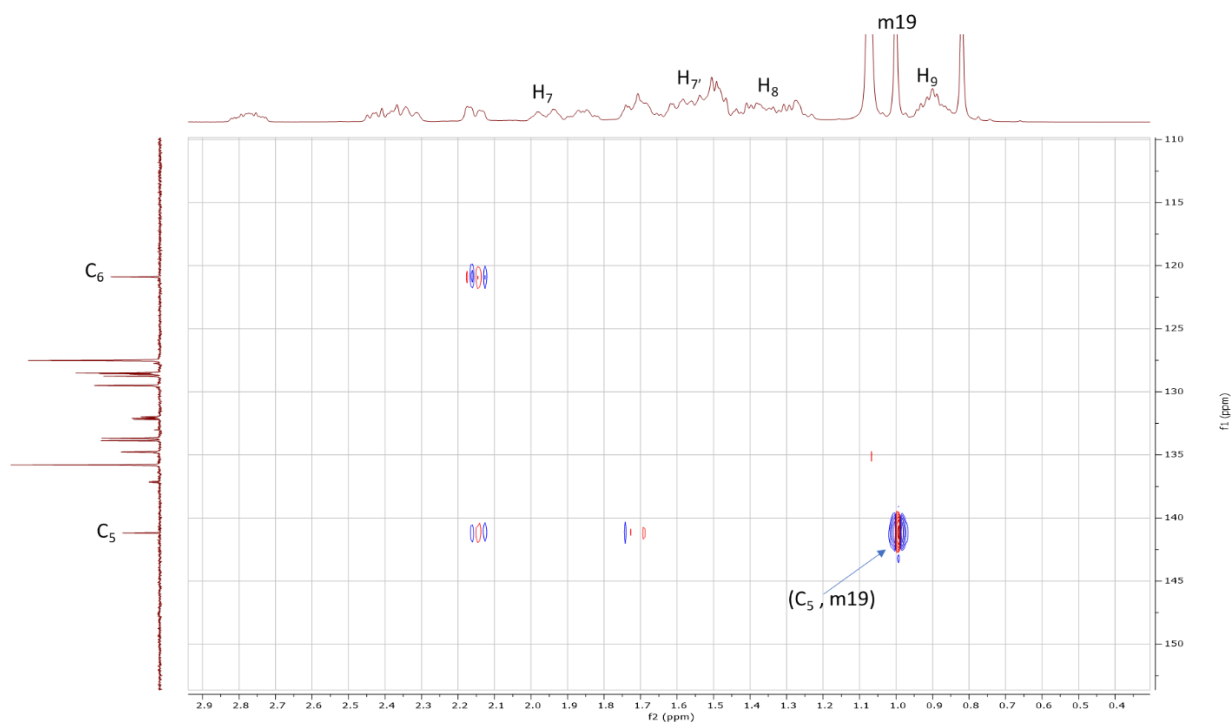
Figure 3.38E ^1\text{H} - ^{13}\text{C} HMBC Correlations in B ring for DHEA \text{C}_{17} Iodide PG (6) ( \text{C}_5 - \text{C}_6 )
