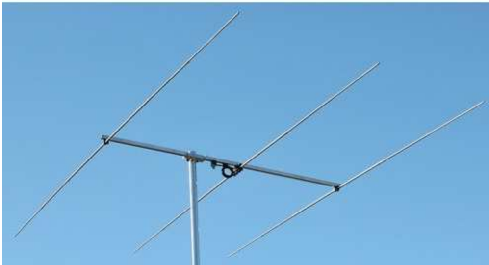
Figure 4-1: Three-element Yagi antenna that operates at 50 MHz. The length of longest element is 3.1 m [80].
