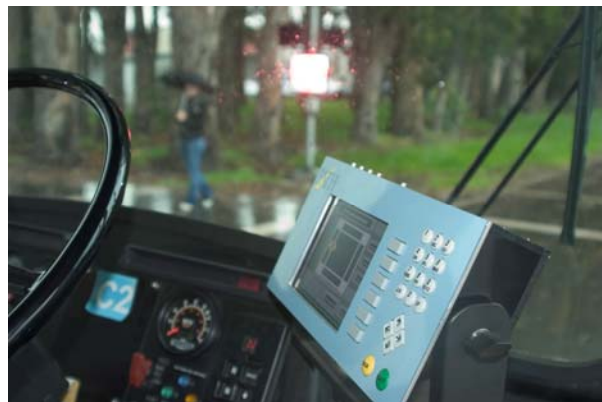
Figure 5.8 View of DVI from Inside the Bus, with the Illuminated DII Ahead
