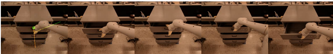
Figure 3.9. Example of retry behavior. The first image is the trajectory sketch generated from the CaP overlaid on the initial observation. The remaining images show the rollout. The robot first attempts to open the drawer by grasping its handle, but fails (2nd image). Then, it retries to open the drawer by grasping the edge instead.
