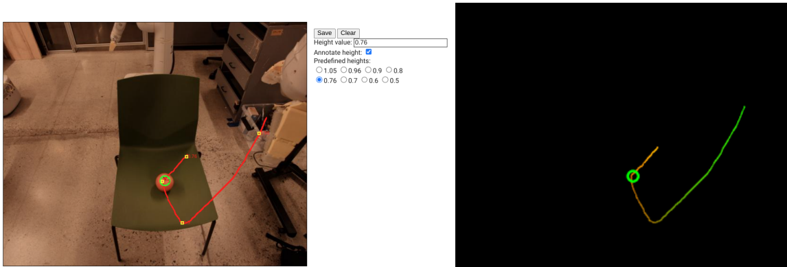
Figure 3.17. Left: The GUI for users to draw trajectory sketches given the robot’s current camera image. The 2D trajectory is directly drawn by manual input, which can then be annotated with interaction markers or waypoints corresponding to user-specified heights. Right: The resulting height-aware trajectory sketch generated according to the output of the UI.
