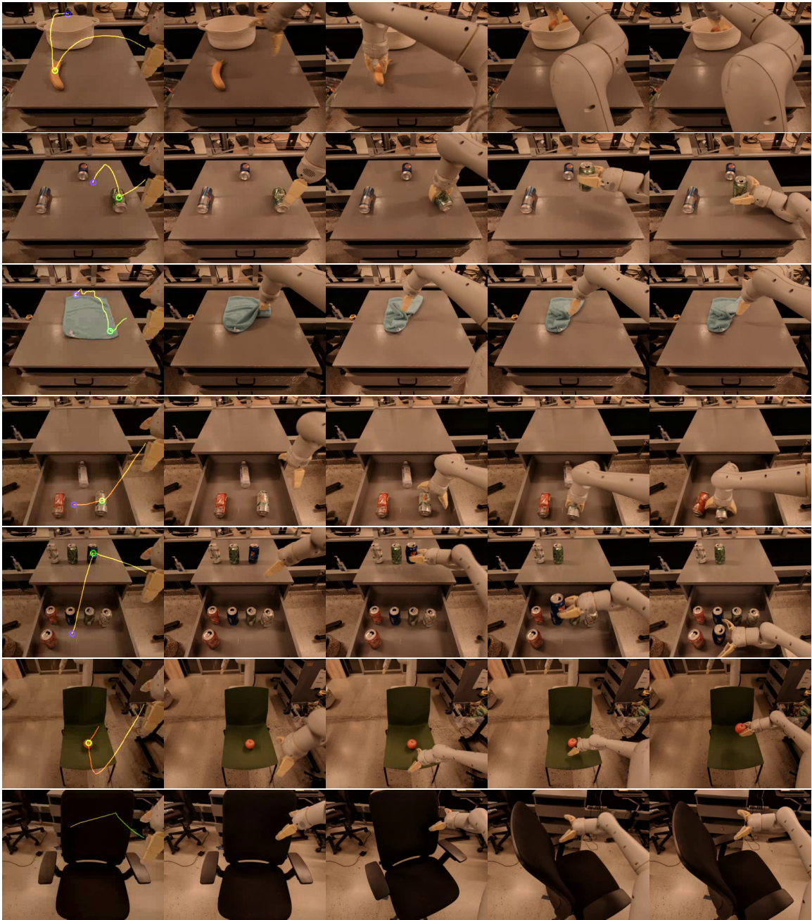
Figure 3.18. Example rollouts of 7 unseen skills. The trajectory sketch overlaid on the initial image is visualized. From top to bottom: Place Fruit, Upright and Move, Fold Towel, Move within Drawer, Restock Drawer, Pick from Chair, Swivel Chair.
