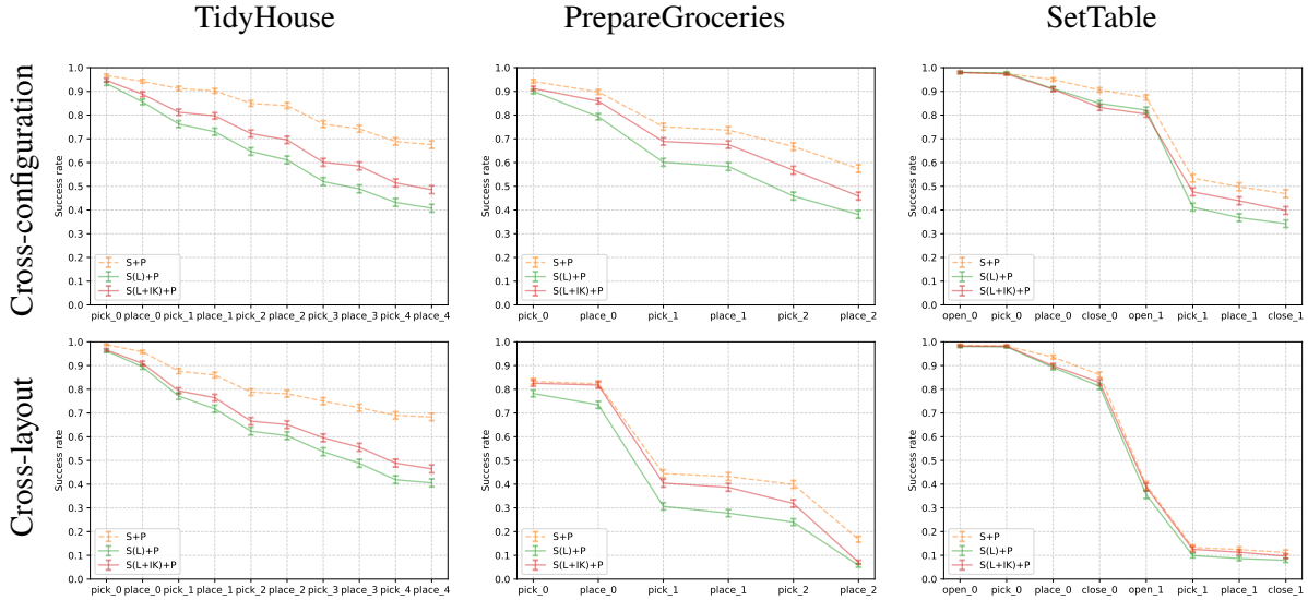
Figure 4.7. Progressive completion rates for HAB [109] tasks. The x-axis represents progressive subtasks. The y-axis represents the completion rate of each subtask. Results of ablation experiments are presented with solid lines. The mean and standard error for 100 episodes over 9 seeds are reported.
