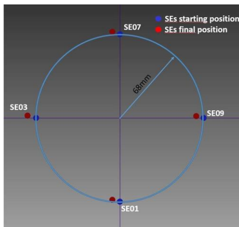
Figure 11: position of the SEs used for tip-tilt and focusing alignment of the AM, as seen from in front of the GWS entrance. The SEs were initially positioned on a cross pattern (blue circles) on a circle 68mm in radius, centered on the nominal center of the GWS focal plane. The pupils we got in these positions were highly defocused, so we moved the AM in focus, tracking the beam at the same time with the SEs. The red circles represent the positions of the SEs where we had, at a visual inspection, pupils with no defocus signal. The final positions of the SEs are shifted, on average, of 6mm in X axis and 2mm in Y axis wrt the starting position
