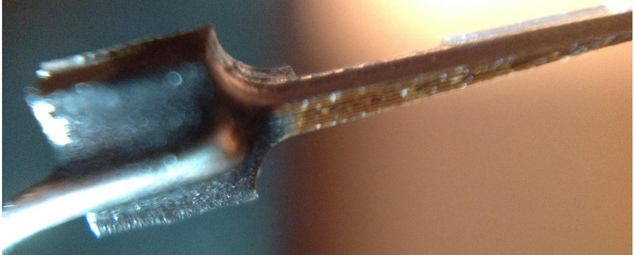
Figure 7. A closer view of the neural probe attached to a wire with a conductive adhesive.
