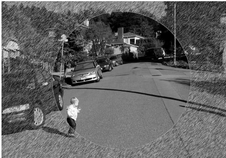
At 50 Km/h the driver begins to see things at the road edges in the background
