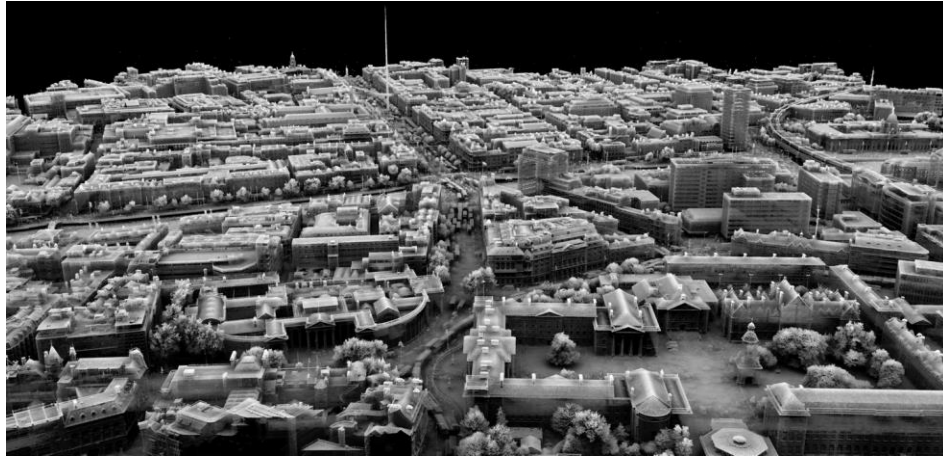
Fig. 2. Dublin LiDAR data seen in 3D looking northward from Westmoreland street, across the Liffey River and up O'Connell street. Digital rendering by Brittney O'Neill and Debra Laefer, 2017.
