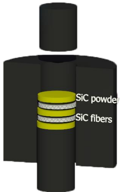
Figure 4. (a) A schematic depicting the main components of a current-activated, pressure-assisted densification (CAPAD) equipment s. (b) A picture of a CAPAD apparatus during an experiment. (Garay, 2010)
