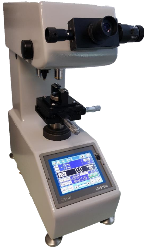
Figure 18. Picture of LECO LM810AT microhardness testing unit.
