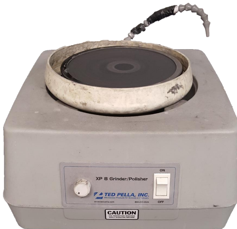
Figure 23. Picture of the grinding and polishing machine used to prepare the SiC samples.
