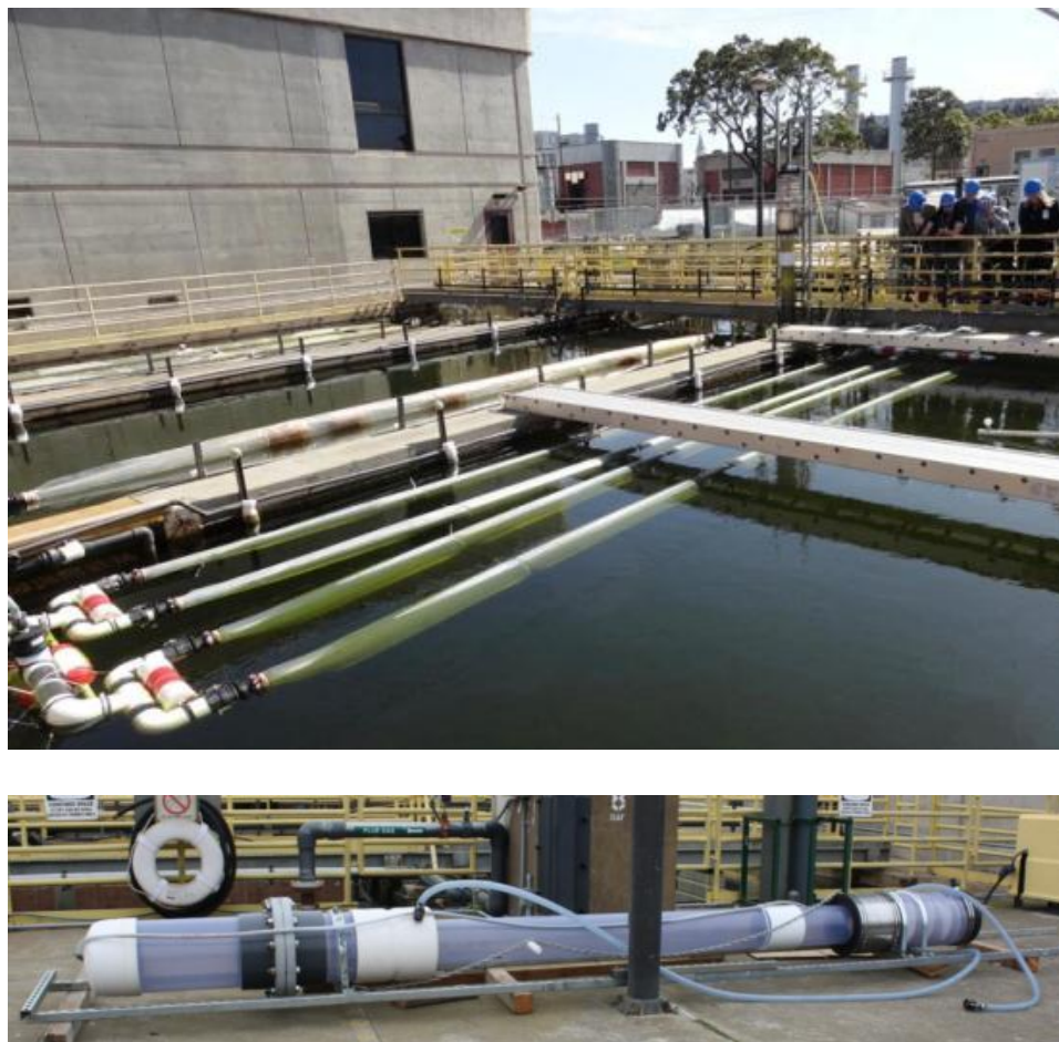
Figure 4.1. The 1500-liter OMEGA system deployed at the SF SEP. (Top) The system consisted of four PBR tubes 10 m in length connected to a centrifugal circulation pump. (Bottom) A scaled version of the GEHC was constructed for supplemental CO 2 injection and as a harvesting location.
