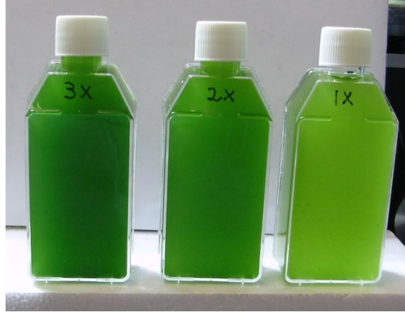
Figure 2.1. Microalgae grown in FPE wastewater following nutrient concentration using an FO membrane. The 1X flask contains FPE that was not concentrated, while 2X and 3X have nutrient concentrations that were doubled and tripled, respectively. The increasing cell density due to higher nutrient availability is evidenced by the darker color of the flasks.
