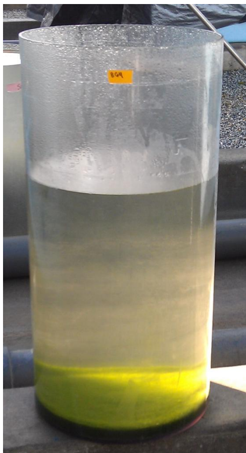
Figure 4.15. Sedimentation of microalgal biomass after being subjected to an EC harvest cycle. When used with a GEHC, the dense microalgal mat will be removed, while the clear supernatant is discharged as final effluent.
