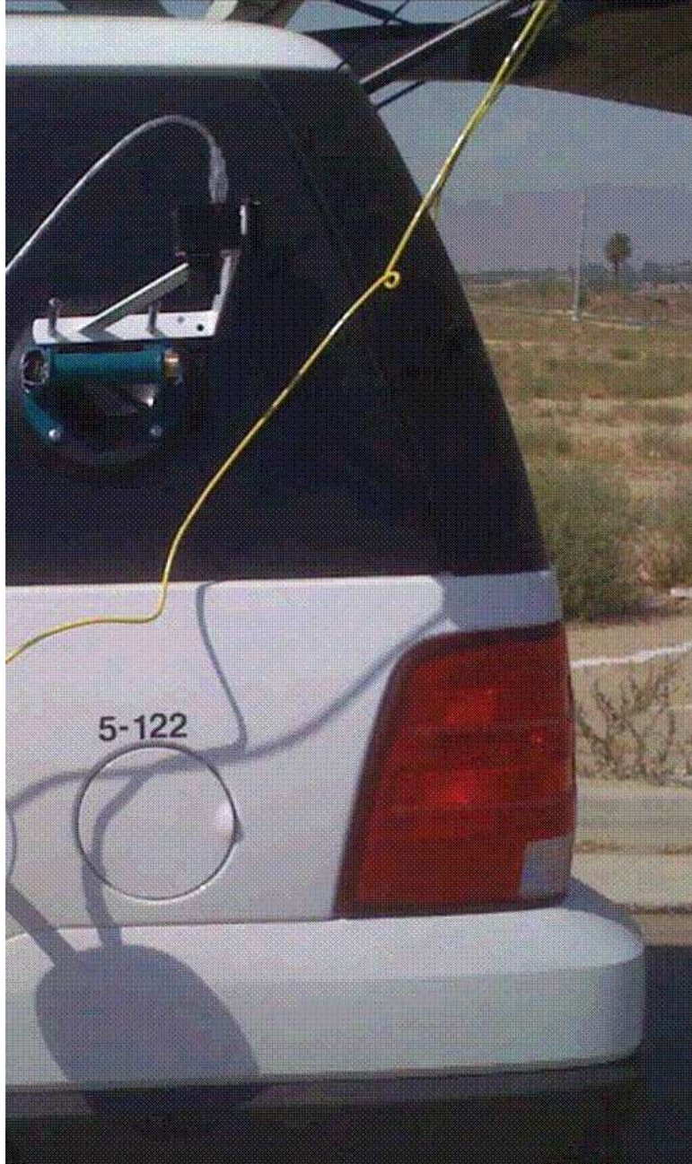
Figure 4-10: Vehicle with mounted vision system for positional accuracy determination.
